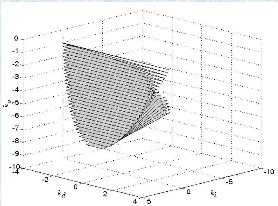
The stabilizing region of  $(k_p, k_i, k_d)$  values for the PID controllers.
