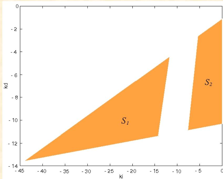
The stabilizing set of  $(k_i, k_d)$  when  $k_p = -18$
