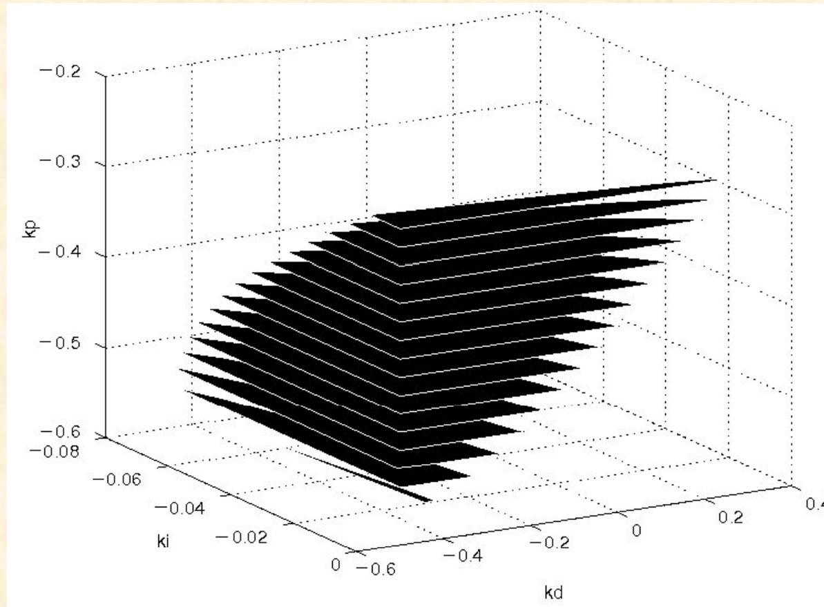
The set of stabilizing  $(k_p, k_i, k_d)$  values for which
