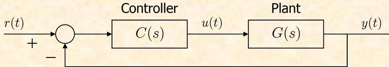
$$G(s) = \frac{N(s)}{D(s)}, \quad C(s) = \frac{sk_p + k_i + k_d s^2}{s(1 + sT)}, \quad \text{for } T > 0$$
