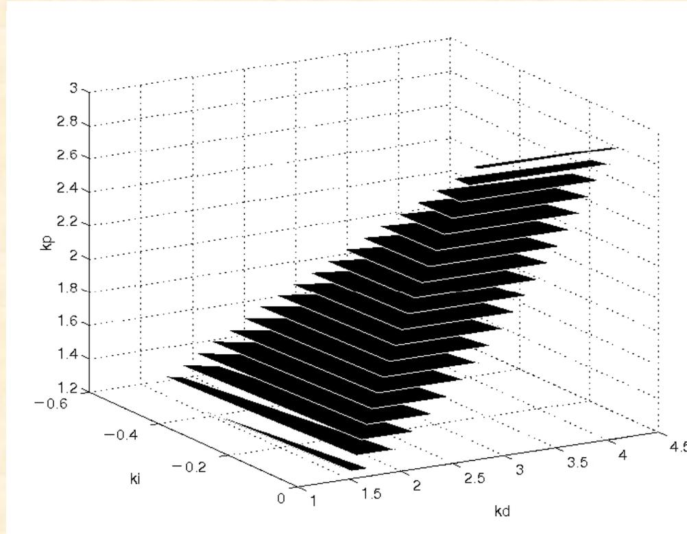
The set  $(k_p, k_i, k_d)$  values for which the resulting closed-loop system achieves a gain margin greater than 3.0 and a phase margin greater than 40 degree.
