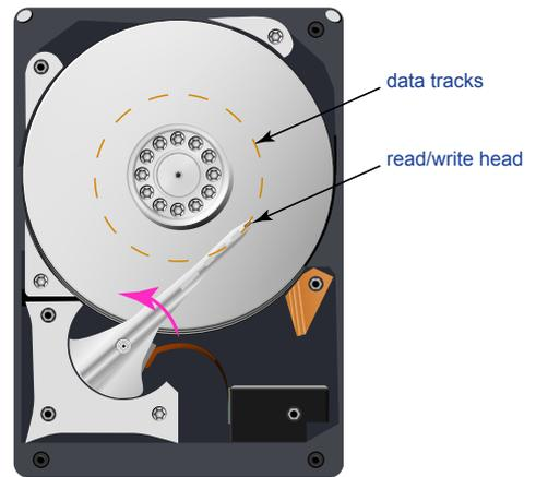
Two sub problems exist for general HDD motion control. First, the actuator needs to provide fast and precise (nm-level accuracy) positioning of the read/write head when switching over different tracks. This transition between data tracks is called “track seeking”. The second problem is called “track following,” which maintains the read/write head over a particular track in the presence of various disturbance signals.
