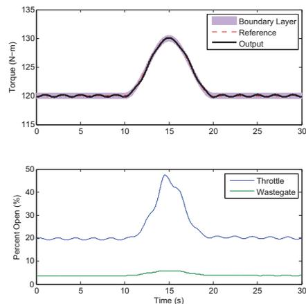
Torque control via throttle and wastegate.
