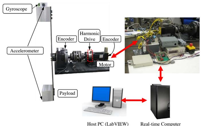
Single joint indirect drive robot setup
