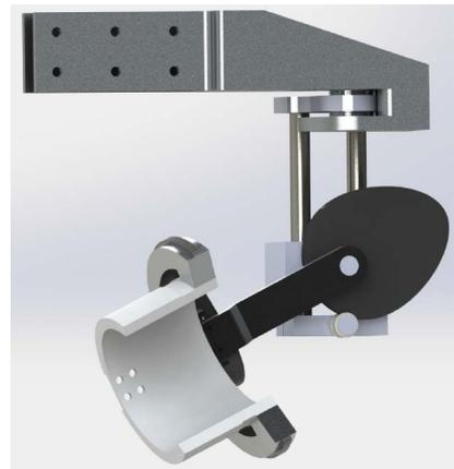
A mechanism was designed which uses a cam to more closely follow the vertical motion of the shoulder
