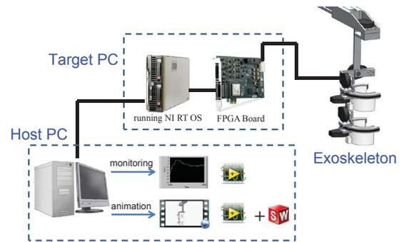
Structure of the real-time data acquisition system (exoskeleton, encoders; target PC, LabVIEW Real-time and FPGA modules; host PC, LabVIEW and SolidWorks.)
