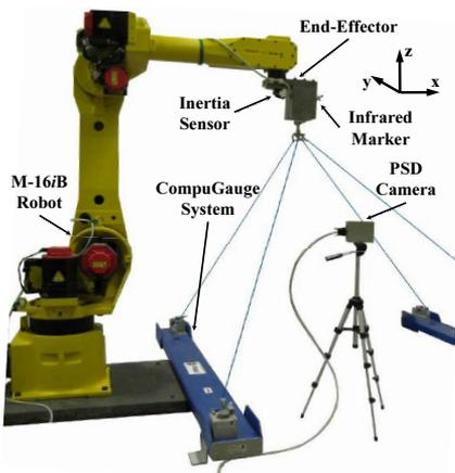
FANUC M-16iB robot system
