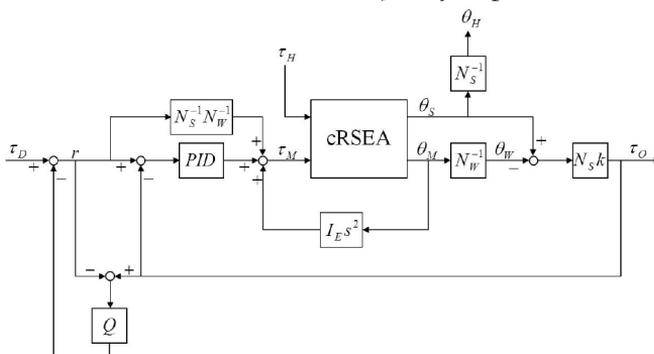
Left: block diagram of the controller for cRSEA;
