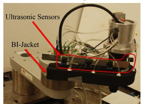
Two-link robot with the BI-Jacket and an array of ultrasonic sensors
