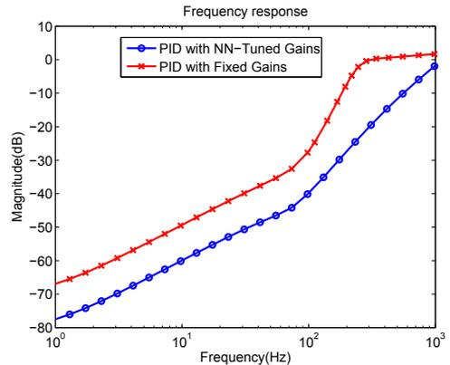
Simulation results of disturbance reduction (piecewise sinusoidal disturbance) and the equivalent sensitivity functions
