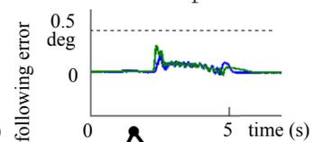
Following error is reduced by applying model-based dynamics and disturbance compensation.
