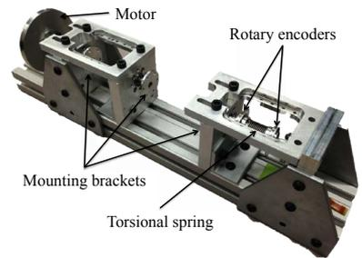
Test rig for VSA position and torque measurements
