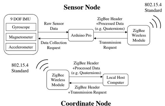
Structure of the wireless joint angle sensor
