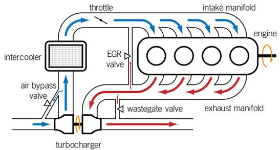
Engine model schematic
