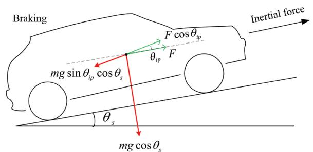
Ideal attitude motion of a vehicle turning on banked circular road and travelling on the slope
