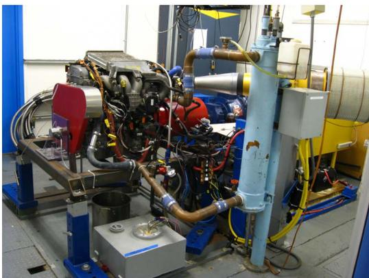
Turbocharged engine test bench
