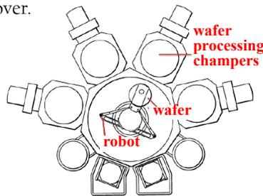
The wafer handling robot inside an IC fabrication tool
