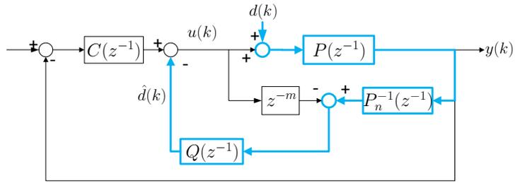
Generalized disturbance-observer scheme for vibration rejection
