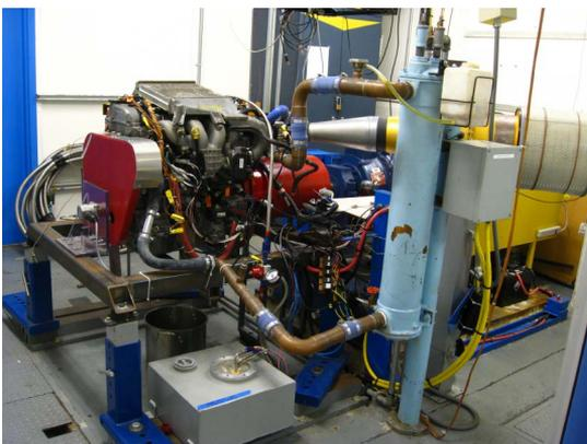
Turbocharged engine test bench
